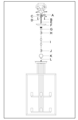
Line art shown may not exactly match the fixture enclosed. However, the installations do apply to this fixture. ITEM NO: 456-8BN-BK 456-80BR-BRZ
